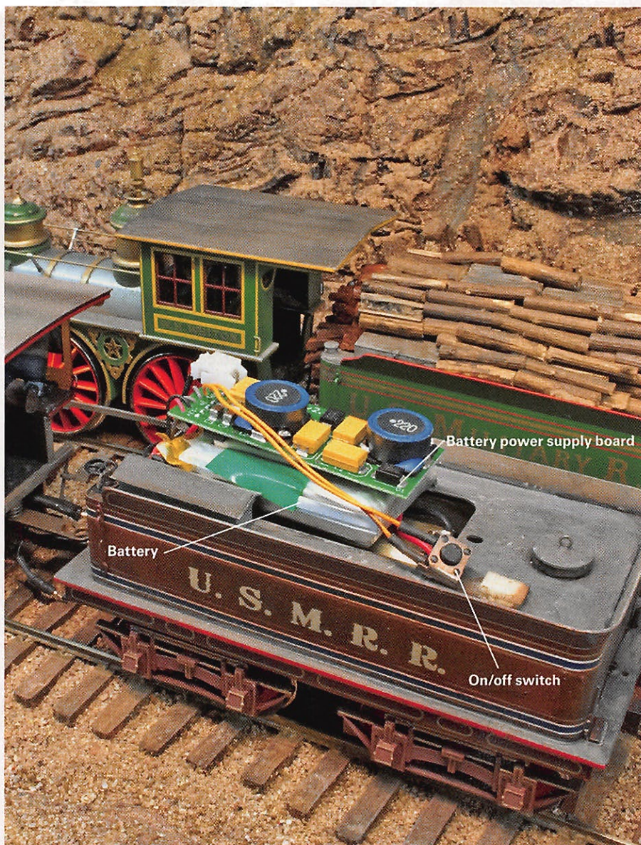
Fig. 6 S-Cab installation. Bernie installed the battery power supply control board with an on/off switch on top of the battery pack. Below that is the sound decoder and radio receiver. The speaker is in the locomotive boiler.
