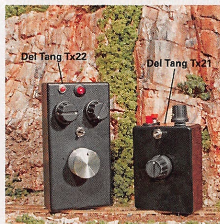
Fig. 3 Del Tang controllers. The Del Tang Tx22 controller can be programmed to store up to 12 different switch-selectable locomotive addresses. The Del Tang Tx21 can only store a single address at a time.
