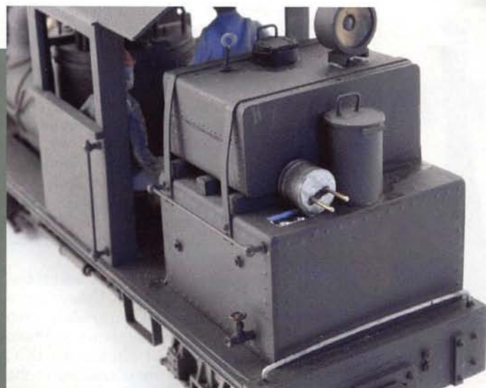
Photos 6 and 7: Here a bridge switch has been disguised as an oilcan on this On3 Shay.
