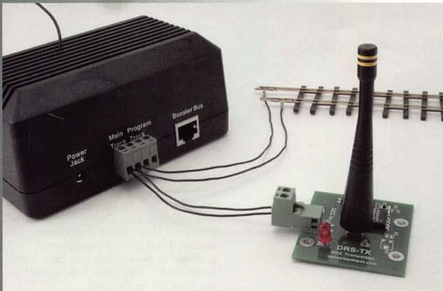
Photo 3: This power supply has been hooked to a Tam Valley DRS-1 system and directly to the track so track-powered DCC locomotives and RC battery-powered locomotives can be operated simultaneously.
