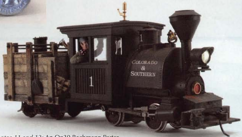
Photos 11 and 12: An On30 Bachmann Porter with a tender for the DRS-1 and battery. The tender can be connected to any DCC decoder.
