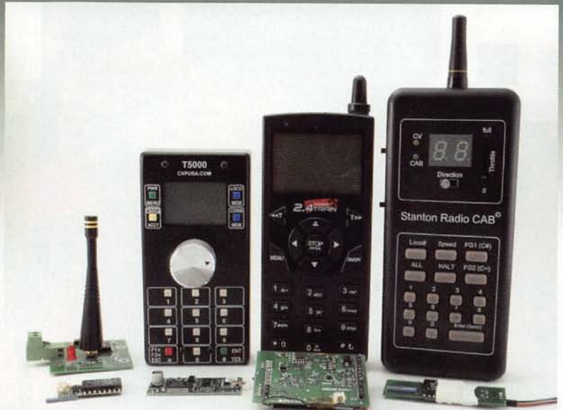
Photo 1: From left to right: transmitters with receivers in front of them. Tam Valley Depot DRS-1, CVP T5000, Aristo-Craft Revolution, and Stanton Radio Cab.
