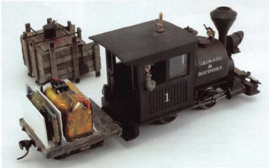
Photos 11 and 12: An On30 Bachmann Porter with a tender for the DRS-1 and battery. The tender can be connected to any DCC decoder.
