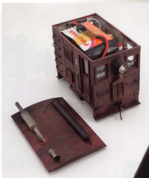
Photo 14: The original Tsunami Sound Decoder was removed from this Blackstone HOn3 K-27 to make room for the Stanton receiver and battery.
