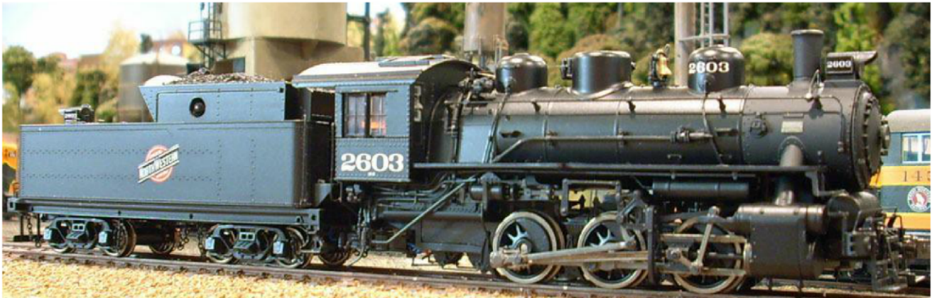
This is an HO Scale switch engine that Bill Pistello converted to battery power. This was one of his first conversions. The system Bill used communicates with the locomotive using infra red light like your TV remote. The system requires the “eye” in the side of the tender which must be able to receive the light signal. This location was rather unsightly and since this locomotive was converted Bill has had some good results mounting the “eye” in the cab window or a tender dog house window where it does not show as much.
