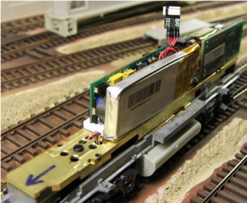
Bill Pistello and his friend, Larry Naus, like to convert models to battery power. Larry converted this HO Scale GP-15 to battery power with this set up. The battery is on the near side wrapped in the silver color.
