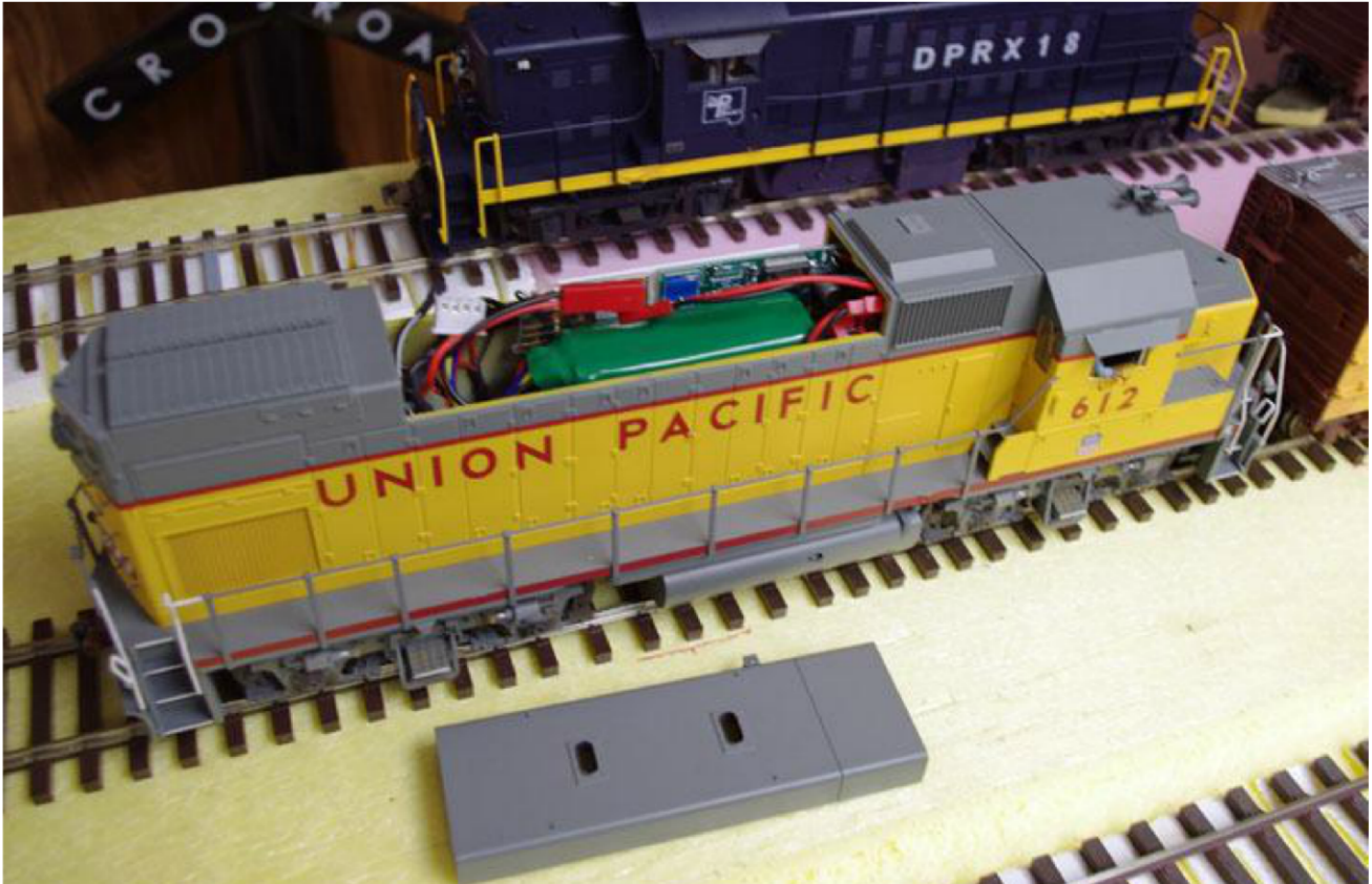
Bill Pistello converted this Atlas O Scale GP-15 to battery power. The green block is the battery.
